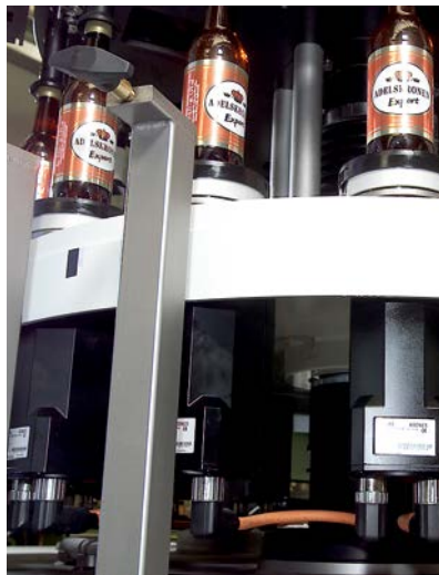
Container table with servomotors, protection type IP65
