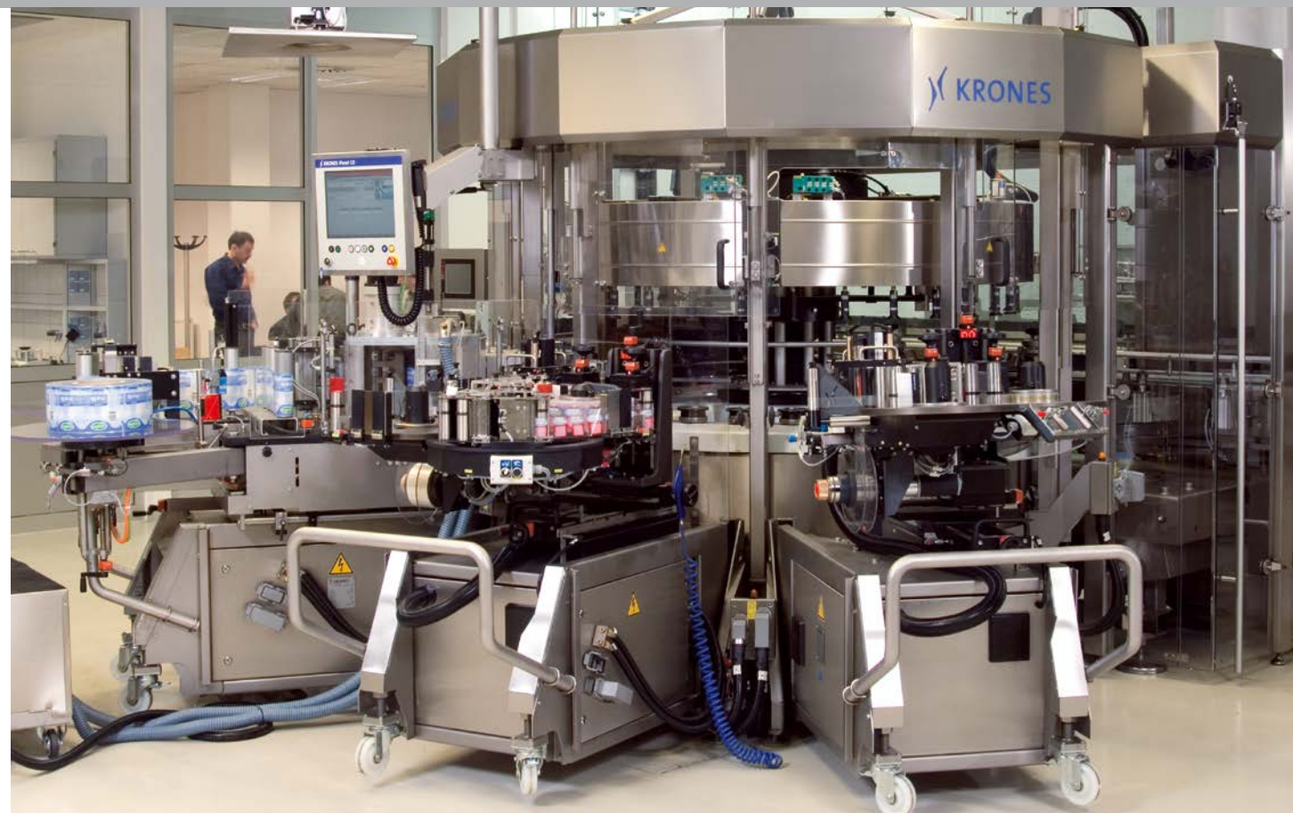
Topmodul with one Controll labelling station (left) and two self-adhesive labelling stations
